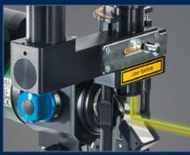
Laser coupling with maximum safety: Mirror based beam combiner with coaxial delivery to the slit lamp.
